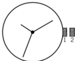
1. To start time-keeping, rotate the crown clockwise 15-20 times in position 1.
